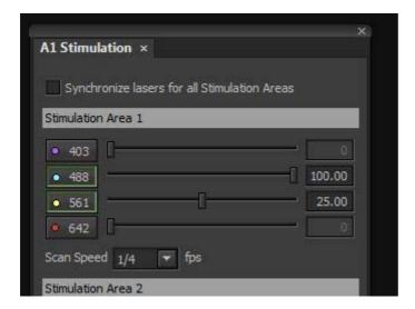
Any combination of available lasers can be used for sequential stimulation. In this example the 488nm and 561nm lasers have been selected. The 488nm laser has been set to 100% power, and the 561nm to 25% power. As there is only one ROI, only Stimulation Area 1 has been set up. The scan speed has been set to 1/4fps, meaning each pass of the laser will take 4 seconds.
