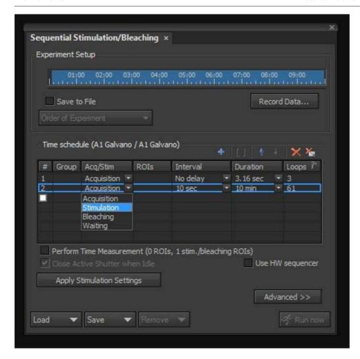
The Sequential Stimulation window looks much like a normal ND Timelapse window. The timeline at the top shows a summary of the experiment. The experiment can be saved directly to disk by selecting the <Save to File> option and specifying a filename and directory. The experiment is divided into phases. These phases can be Acquisition, Stimulation, Bleaching or Waiting.
