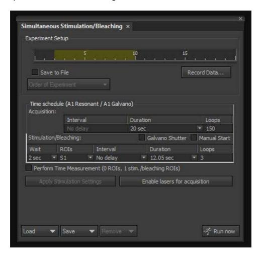
Once the ROI, laser settings and experiment phases have been set up, click <Apply Stimulation Settings> to prepare the experiment. If you move the ROI you will need to click <Apply Stimulation Settings> again to prime the experiment.
