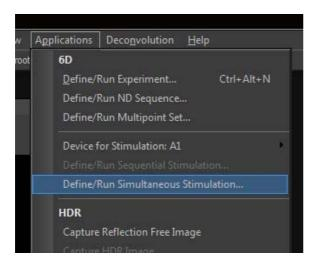
The Simultaneous Stimulation window looks slightly different from the Sequential Stimulation window. The experiment is set up as a continuous no delay acquisition, and then the stimulation/bleaching phase is "nested" within this acquisition.
