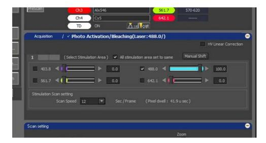
Here the different stimulation groups are displayed as tabs rather than expanded panels. The <All stimulation area set to same> option is also available. This panel contains laser lines, powers and scan speeds. In this GUI, however, the scan speed is shown in **seconds per frame** e.g. a scan speed of 12 sec/frame will mean that a single pass of the stimulation laser will take 12 seconds, whereas a speed of 1/16 sec/frame means a single pass will take 1/16 of a second.
