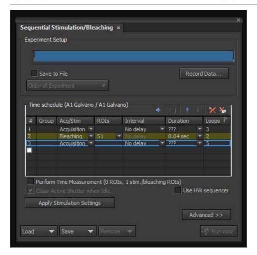
The scan speed is the time taken for the laser to pass from the top left pixel of the bounding box of the ROI to the bottom right pixel. In a rectangular ROI the laser will be on for the full scan speed time. For other shapes of ROI, for example irregular Bezier shapes, the scanner will zoom to the smallest possible box surrounding the shape and then use the AOTF to turn the laser on and off, so stimulation light only hits the desired regions.
