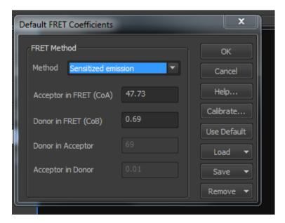
Once you have the calibration, simply collect your sample image again using the two OCs. Then under Applications select FRET view.
