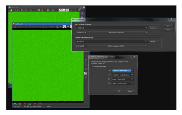
Capture the an image with donor only and one with acceptor only using the two OCs created previously. Then select Applications> FRET calibration to get the pop up window shown above. With the images open you can select the open files from the drop down menu that relate to the Donor only and acceptor only image. You can draw ROIs in the images to better show the regions of sample too. It is recommended to set a background ROI too.
