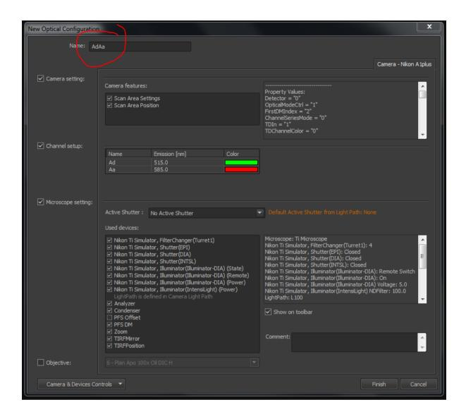
Then image your control samples and main sample by setting up an ND acquisition with the two OCs selected in the wavelength tab
