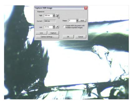
6) Repeat this process for the Low exposure setting so that the live image looks dark but contains detail using the "Low" input field Low 10 ms and corresponding arrow button .
